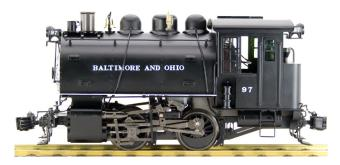
AML is proud to offer the famous B&O "DOCKSIDE" of the Baltimore Waterfront. Four switchers were built in 1912 by Baldwin for the B&O. Initially constructed as saddle tank engines, some were given tenders in later years. The diminutive size and short wheelbase were required to handle the tight curves of these lines.
